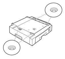
4 Place the machine over the tray, aligning the feet on the machine with the positioners in the optional tray.
